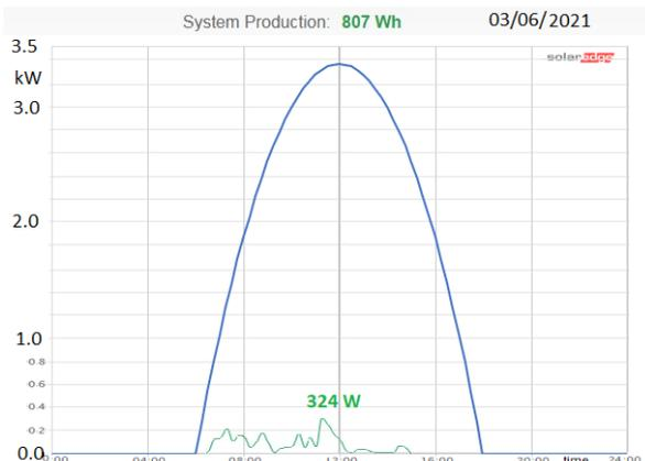
This day had a peak output electric power of only 324 W (one-tenth of the normal peak) and the lowest energy of 807 kWh, a significant reduction of 97%,
