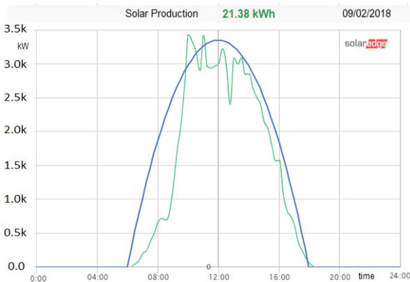
Figure 10 shows a partially cloudy morning, and improper declination which have given rise to a 30% reduction in power output.
