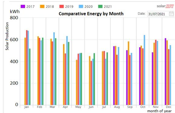
The pattern of monthly energy production is seen to be somewhat consistent for the same month over the 4 years, but with reductions caused by the declination angle and the orientation of the solar panels. It is worthy to note that the reduction occurred in certain months as the solar panels were fixed and not rotated to capture maximum of the Sun's direct rays.
