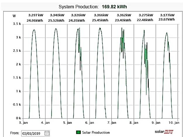
It is observed that during this week, the peak power is constant at around 3.3kW, but the production of energy varied a little between 22.5 kWh and 25.5 kWh, with a total weekly production of 169.8 kWh.
