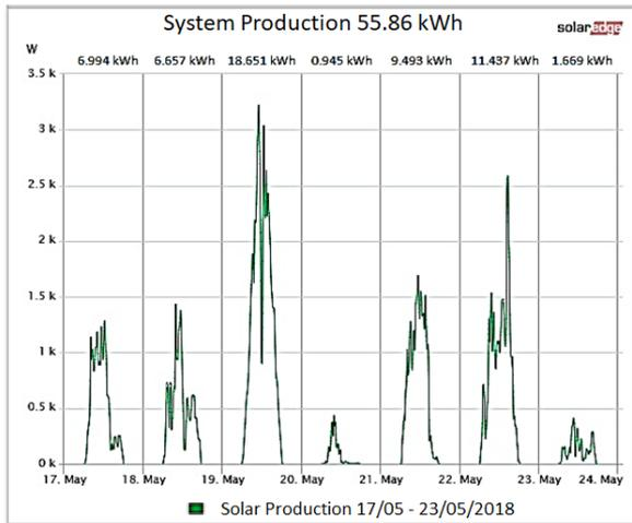
The corresponding output of electrical energy varied substantially from day to day, between 0.94 kWh and 18.65 kWh. As planning for such weeks is quite complex, it is important to know how often such days or weeks occur. This issue is addressed in this paper.
