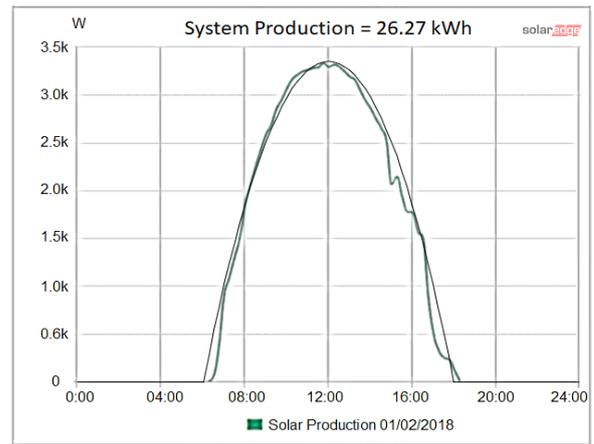
The recordings on this day on the monitoring portal show a peak power production of 3.332 kW and an energy of 26.27 kWh for the day. These values correspond very well with the earlier predicted maximum values of 3.328 kW and 26.5 kWh/day.
